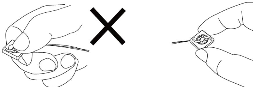
**Don't pull fan with lead wires.**
