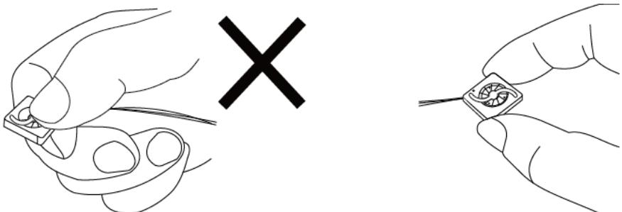
**Don't pull fan with lead wires.**
