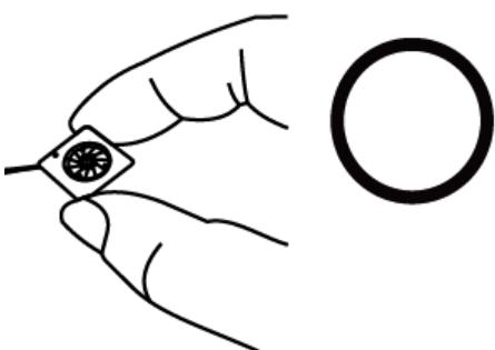
**Don't pull fan with lead wires.**
