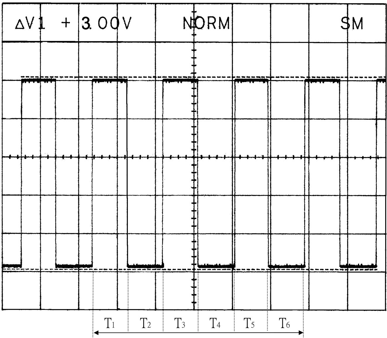
$$T = T_1 + T_2 + T_3 + T_4 + T_5 + T_6 = (1 \text{ Rotation})$$
