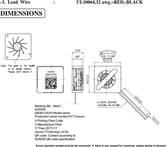
About recommend connector, SUNON recommend the following models for SUNON Mighty Mini Fan/Blower: 1.(JST) SUR series connector: 02SUR-32S / 03SUR-32S / 04SUR-32S.
