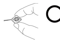
Don't pull fan with lead wires.
