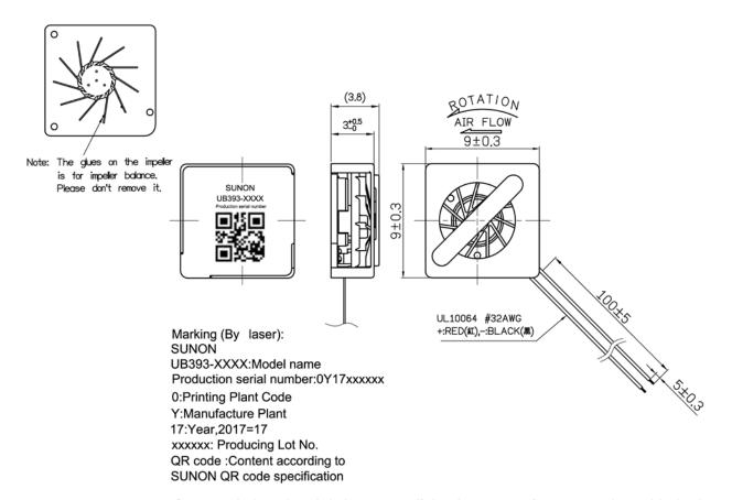
Sunon standard sample exclude the connector. If there is any request for connector, please advise in advance. About recommend connector, SUNON recommend the following models for SUNON Mighty Mini Fon/Blower: 1.(JST) SUR series connector: 02SUR-32S / 03SUR-32S / 04SUR-32S.
