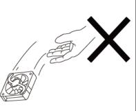
Don't cut the fan or lead wires
