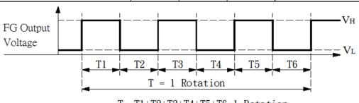
T= T1+T2+T3+T4+T5+T6=1 Rotation  $T = \frac{60}{\text{rpm}}$
