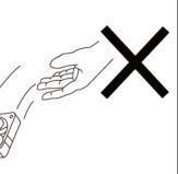
Don't cut the fan or lead wires
