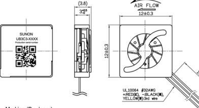
Marking (By laser): SUNON UB3C3-XXXX:Model name Production serial number:0Y17xxxxxx 0:Printing Plant Code
