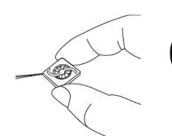
Don't pull fan with lead wires.
